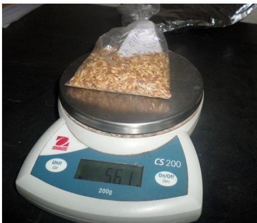
Plate 3.1: Measurement of seed impurities using an electronic balance
